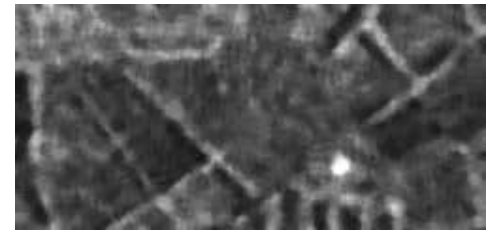
Speckle reduction using an averaging filter
