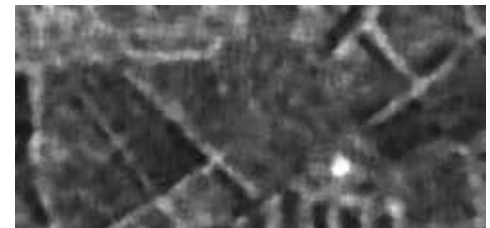
Speckle reduction using an averaging filter
